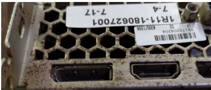
Serious rust caused by humidity
